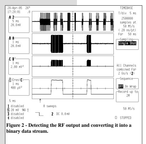
The detection scheme used in the measurement of the rf pulse risetime can be used to detect the entire data packet. Figure 2 shows how this can be done.
